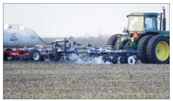
Figure 6.26. The white cloud seen behind the knife is water droplets that form as ammonia lowers the temperature.
