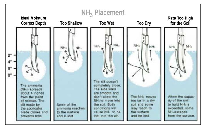
Figure 6.25. Distribution of anhydrous ammonia (white areas) when released in different kinds of soil, at various depths, and under several soil moisture conditions.
