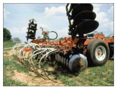
**Figure 6.27**. Application of anhydrous ammonia with a tillage tool saves both time and fuel. This system works well on land which is at the correct moisture for tillage operations.
